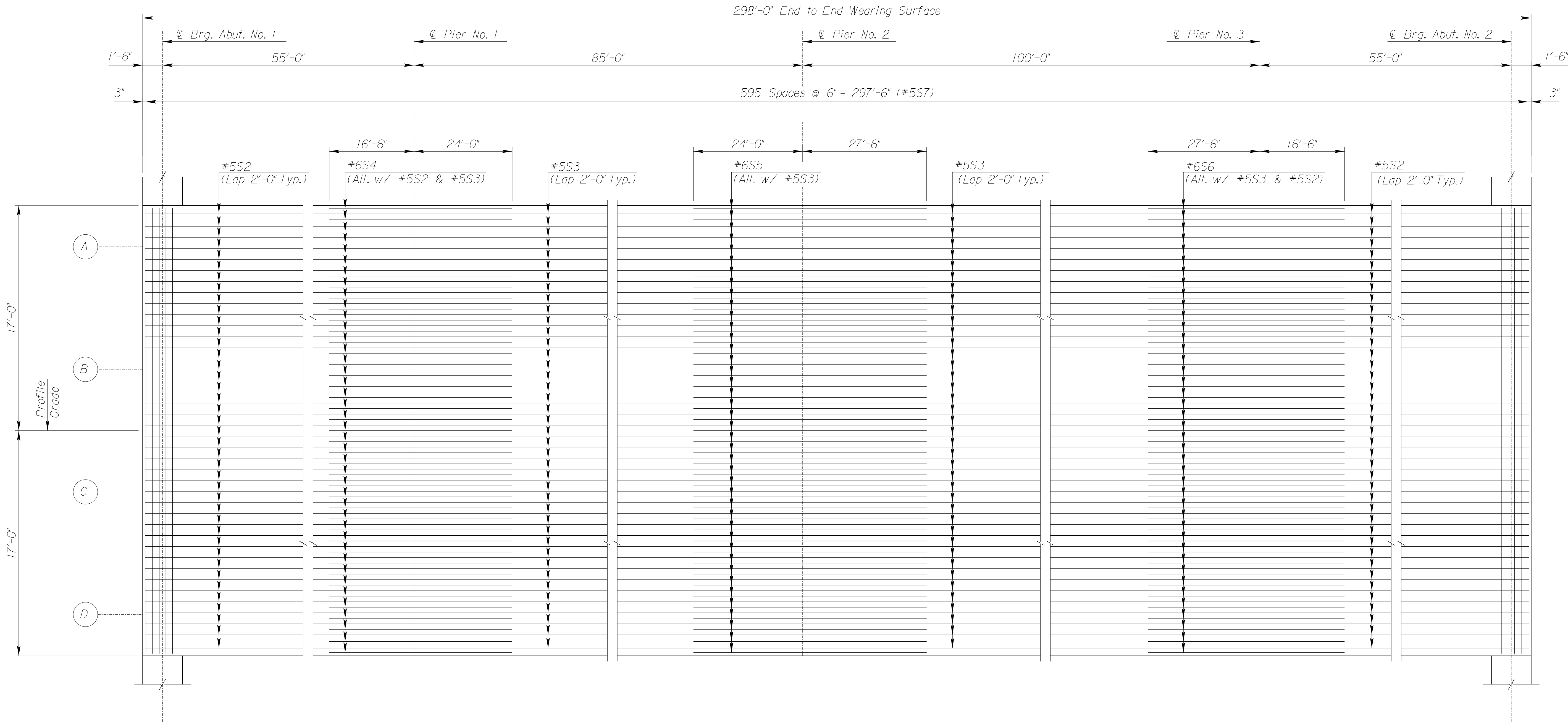
PLAN SHOWING REINFORCING IN TOP OF SLAB NOTE: See Slab Section for spacing of longitudinal reinforcing
